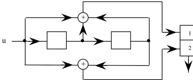
that generates two bit outputs  $v_1, v_2$  for every input bit
