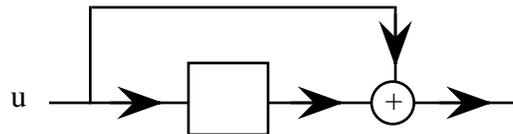
with input  $u = u_0u_1u_2 \dots$  and output  $v = v_0v_1v_2 \dots$  that transmits data in blocks of  $n=1$  with  $k=1$ . Note that the box contains a D flip-flop and as usual the addition is mod (2)
