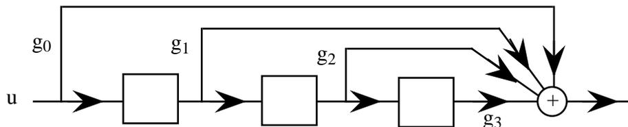
We call this a **linear feed-forward shift register**. The values of the  $g_k$ 's are 0 or 1 depending on whether or not the link is present. Assuming  $g_0 = g_1 = g_2 = g_3 = 1$
