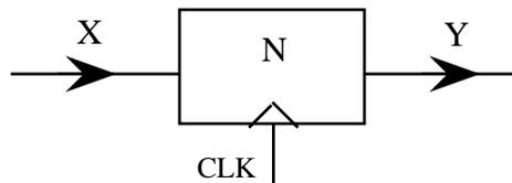
that adds a parity bit to every 8 bits of data. Hint - use an exclusive-or gate.
