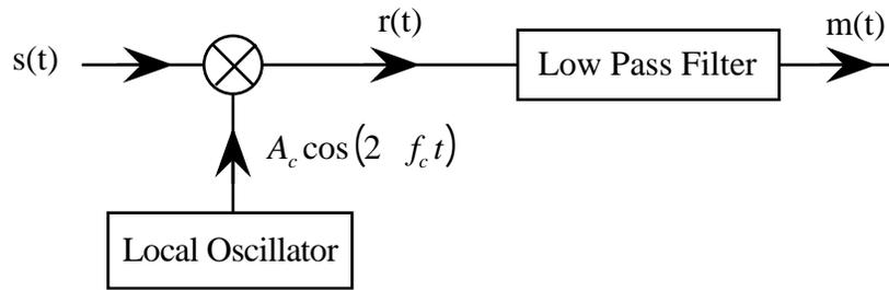
with a local oscillator generating a carrier frequency at the same phase as the transmitter will demodulate the DSB-SC signal with the following spectrum
