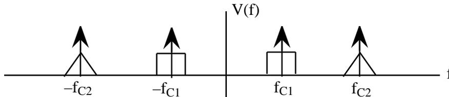
with  $f_{C1} = 600 \text{ KHz}$  and  $f_{C2} = 700 \text{ KHz}$  and that  $f_{LO} = 1.155 \text{ MHz}$
