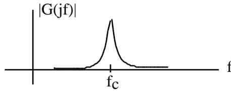
with an adjustable center frequency  $f_c$ . But this is hard to do. A more practical circuit is a **superheterodyne** - or **superhet** as follows
