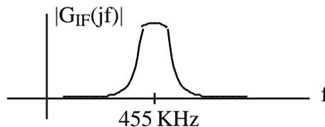
with a passband that is wide enough for only one radio station. Note that we refer to  $f_c = f_i = 455$  KHZ as the **intermediate frequency (IF)** and the passband filter as the **IF Filter**. Note that the "carrier frequency" of the radio station that makes it through the bandpass filter has been shifted to  $f_c = 455$  KHZ
