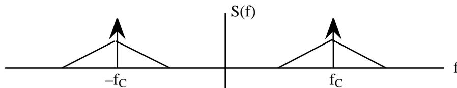
6. The objective of this and the rest of the problems of this Investigation is to introduce some variations on amplitude modulation that reduce the power and bandwidth of the modulated signal at the expense of circuit complexity. The first is Double Side Band–Suppressed Carrier modulation which is referred to as DSB-SC. DSB-SC is just like AM except that the carrier sinusoid is not transmitted as indicated in the following spectrum of a DSB-SC signal
