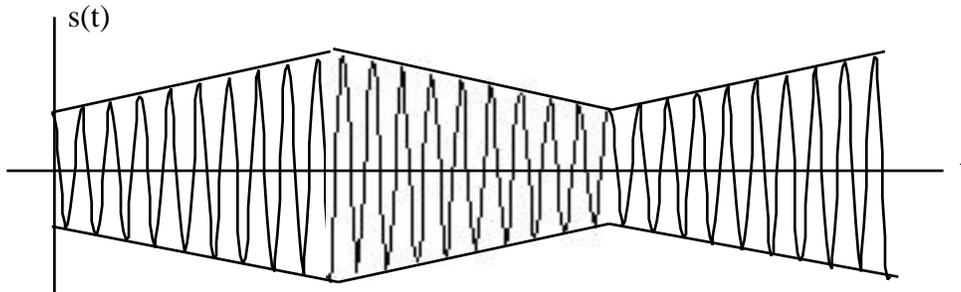
from all those being received by the antenna we need to demodulate it - recover the baseband signal  $m(t)$ . One relatively simple way to do this is with an **envelope detector** as follows
