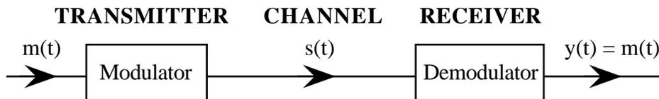
consisting of a transmitter, a channel like space or fiber optic and a receiver.
