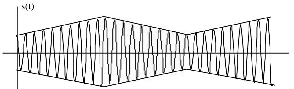
are referred to as the **envelope** of the amplitude modulated signal.
