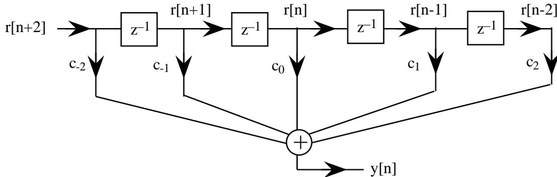
Note that the  $c_k$ 's are the impulse response of the FIR filter
