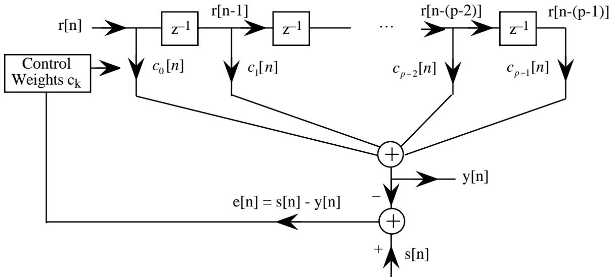
Now to actually implement the LMS algorithm the equalizer needs to know the signal  $s[n]$  being transmitted in order to calculate the error  $e[n]$ . So before sending any real data the transmitter sends a signal  $s[n]$  that the equalizer knows the value of so it can calculate  $e[n]$ . Note that this must be done every time a new connection is made
