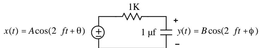
is how the amplitude and phase of the *sinusoidal steady state response* varies as a function of frequency  $f$
