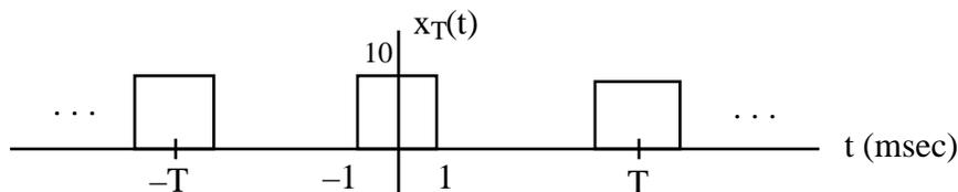
that has a period  $T$  long enough for the circuit's response to for all practical purposes "decay to zero" between pulses
