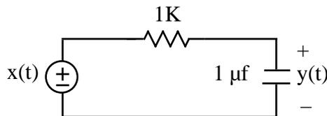
with **zero initial voltage** across the capacitor at time  $t = -10^{-3}$  when the following single pulse arrives
