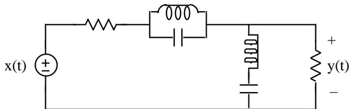
on its pole-zero diagram. Explain how you got your result and then sketch  $|G(j\omega)|$ . Hint - find  $y(t)$  at the resonance frequencies  $\omega_{01}$  and  $\omega_{02}$  of the series and parallel LC circuits.
