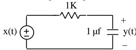
by analyzing the corresponding **Fourier Transformed Circuit**
