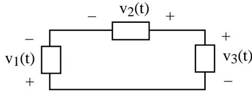
satisfy  $V_1(\omega) - V_2(\omega) + V_3(\omega) = 0$
