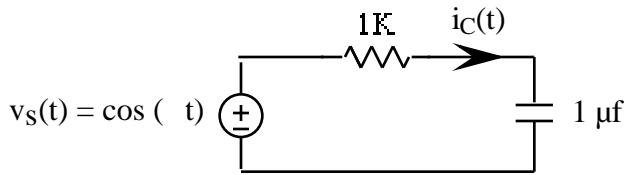
to find how the sinusoidal steady state response of  $i_C(t)$  varies as a function of frequency.
