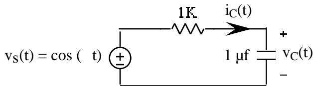
for the sinusoidal input  $v_s(t) = \cos(-t)$ . Now find  $V_C(j\omega)$  and  $I_C(j\omega)$  in terms of the phasor  $V_s$  for the same circuit but with the more general input
