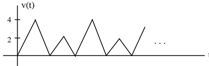
if the trigger level is 3 volts and the slope positive
