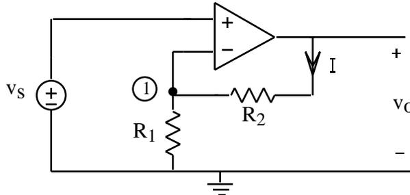
are independent of the op amp gain  $A$  when the op amp is operating in its linear active region. This is particularly nice because it means that  $A$  is not a critical parameter - all  $A$  has to do is be large. This is nice because it makes op amps easier and cheaper to build.
