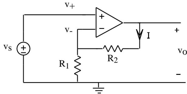
We call this a positive gain amplifier because, as we will show,  $v_o$  is equal to a positive constant times  $v_s$ . Note that we usually don't draw in the power supplies when we draw op amp circuits.
