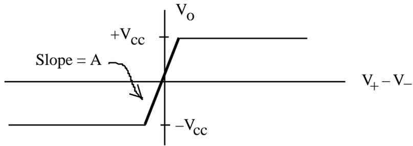
we see that the op amp will go into **saturation** - will reach its maximum value - when  $V_O$  reaches the value of  $V_{CC}$ . The way to determine if an op amp is in saturation is to simply calculate its output voltage assuming the op amp is operating in its linear active region and see what you get. If the linear model predicts  $V_O > V_{CC}$  then the op amp is in saturation with  $V_O = V_{CC}$ . Otherwise it's operating in its linear active region. Assuming  $V_{CC} = 15$  volts
