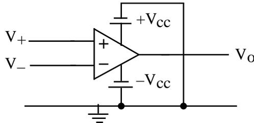
Op amps (powered by DC supplies  $+V_{CC}$  and  $-V_{CC}$  that are typically on the order of 15 volts) are voltage amplifiers characterized by transfer characteristics as follows
