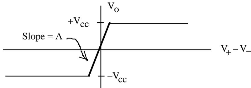
where the output voltage  $V_O$  is a function of the **difference** ( $V_+ - V_-$ ) between the two inputs  $V_+$  and  $V_-$ . As a result of this we refer to op amps as **differential** voltage amplifiers.
