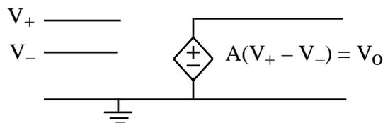
We then say our op amp is **operating** in its **linear region**. Note that no current can flow into the + or – terminals of our ideal op amp model. This is a reasonable approximation to real op amps because they typically have equivalent input resistances of at least 200M.
