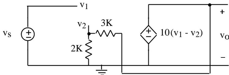
4. The objective of this problem is to illustrate what happens when we connect a load to a circuit containing a controlled source. Suppose we take a resistor circuit containing a controlled source like the following
