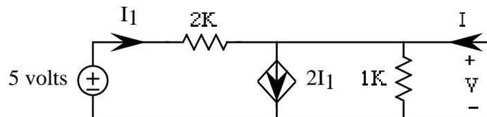
as those not containing controlled sources but resistor circuits with controlled sources also have Thevenin Equivalents. And so we can write
