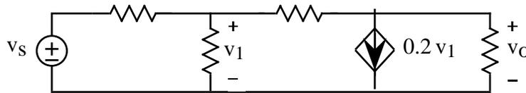
are proportional to the **independent** source  $v_s$  just like they are in resistor circuits not containing controlled sources. The main objective of this investigation is to calculate the Thevenin Equivalents of such circuits.
