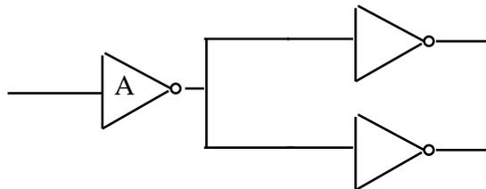
when we include the affects of the "long wires" connecting the inverters. Given that  $R_n = 1K$ ,  $C_n = 5 \text{ fF}$ ,  $R_p = 1.5K$  and  $C_p = 10 \text{ fF}$  and  $R_i = 1K$ ,  $C_i = 2\text{fF}$
