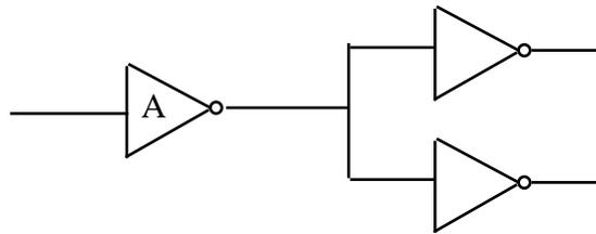
Note that the **fanout** of a logic gate is the most gates it can drive and still meet its specs.
