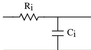
where  $R_i$  is the resistance of the conductor alone and  $C_i$  the capacitance of the capacitor alone. This model is not perfect but at least it gives a reasonable ballpark approximation of what's
