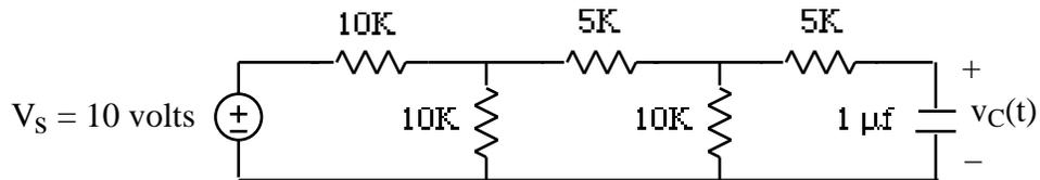
Note that it's straightforward to find  $R_{TH}$  for this circuit without having to write or solve any equations. Be sure to draw the circuit you're analyzing to find  $R_{TH}$
