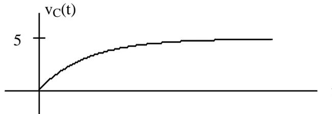
with  $v_C(t) = 5 - 5e^{-1000t}$  getting closer and closer to  $V_S = 5$  volts as the capacitor charges up. Now, this response - like the responses of all such circuits with nonzero inputs - is the sum of two "parts"
