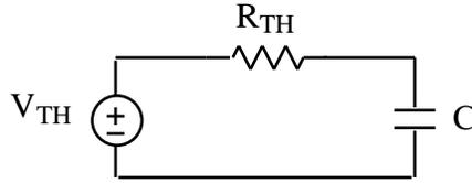
then for such a circuit is equal to  $\tau = R_{TH}C$ . **Memorize** this result for first order RC circuits. Note that most engineers consider transient responses to have decayed to zero by time 5
