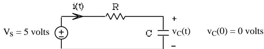
to decay to zero and the circuits reach steady state. Let us begin by **defining** the **time constant**  $\tau$  of such a circuit by
