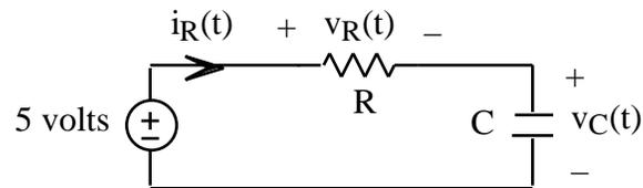
Assuming this circuit has zero initial conditions with  $v_C(0) = 0$  volts
