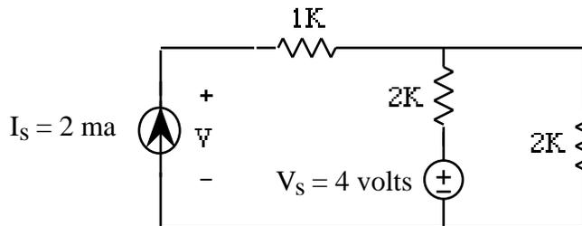
7. Use superposition to find  $V_o$  in the following circuit. Be sure to **draw** the corresponding circuits
