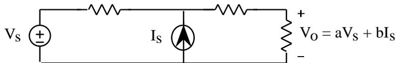
by first finding the response to  $V_s$  when  $I_s$  is set to zero and then finding the response to  $I_s$  when  $V_s$  is set to zero. We refer to this procedure as **superposition**. **Memorize** this result - its important because it says that each source contributes its own independent term to the output. Describe in words how superposition can be used to find voltages and currents in a circuit with n sources.
