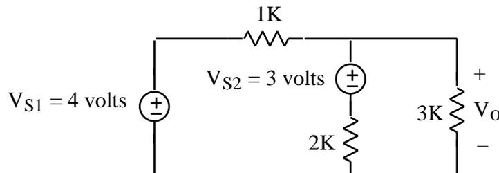
Hint - you can reverse  $V_{S2}$  and the 2K resistor without affecting any voltages or currents in the circuit
