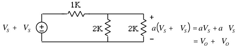
Hint - first redraw the circuit with the single voltage source  $V_s + \Delta V_s$  replaced by a voltage source of value  $V_s$  in series with a second voltage source of value  $\Delta V_s$ . And then make use of superposition to obtain the circuit for finding the response to  $\Delta V_s$
